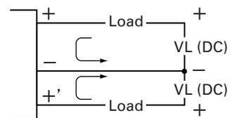
**NOTE :** Sum of continuous load current must not exceed the maximum rating.
