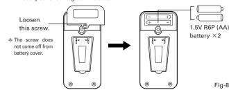
NOTE: Remove the battery when the instrument is out of use for a long time. The exhausted battery might leak electrolyte and corrode the inside.
