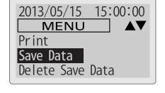
②Confirmation screen as shown in the right is displayed. Select "YES" and press ← (ENTER) Key for saving the test result. Select "NO" and press ← (ENTER) Key for go back to Menu screen (previous Step ①).
