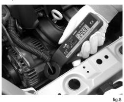
4 Start the engine, and read the measurement value on LCD. **NOTE**: The value should be minus (-) if the current flows opposite direction of "⇒" mark on clamp head.
