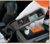
Car Alternator : Engine generator that outputs DC electricity. Measuring its charging current is effective to find the trouble that might cause battery
